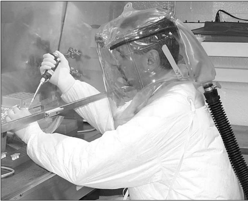
Fig. 4. A worker in a BSL-4 laboratory wearing protective gear. BSL-4, or biosafety level 4, is the highest level of biosafety and is used for diagnosis of high-risk agents.
